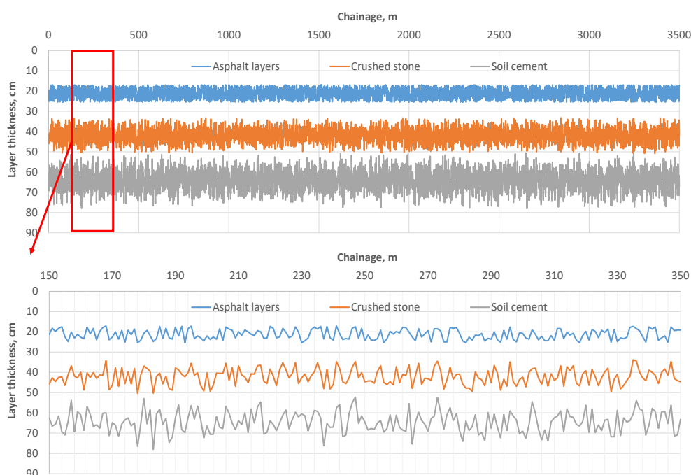
Figure 5. Layer thickness of pavement on nearest traffic line from ground radar test.
