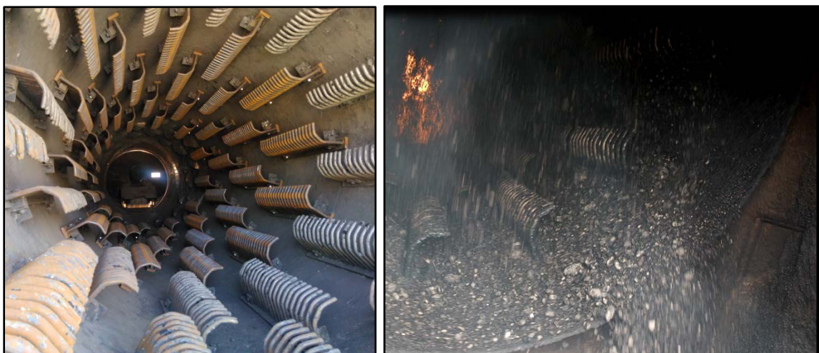
Figure 4. View of the inside of the black drum before and during production.
