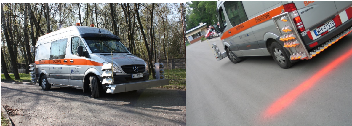
Figure 1. Multifunctional SPDE measuring system for measuring surface characteristics of the pavement and photographic recording of damages.
