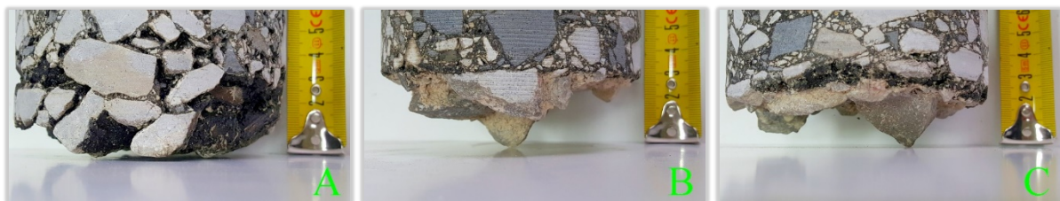
Figure 5. Examples of a complicated shape of the bottom surface of an asphalt layer package leading to significant uncertainty in determining package thickness on a core sample: A) significant losses and deformations due to insufficient bottom compaction, B) a well-defined flat surface partially masked by subbase aggregate grains from underneath, C) large aggregate grains (clearly larger than grains embedded in the package) penetrating the package bottom (clearly immersed in the asphalt mix).
