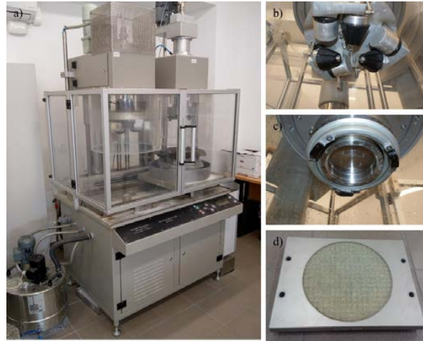
Figure 2. a) The FAP test equipment b) polishing rotary head, c) friction measuring rotary head, d) glass control plate.
