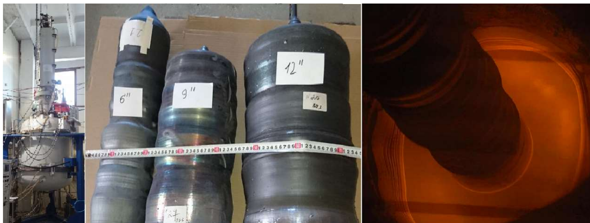
Figure 4. Electron beam pulling process. A- puller (detail description in [15]); B- 6"; 9"; 12" ingots archived on puller shown at A; C- view of process.
