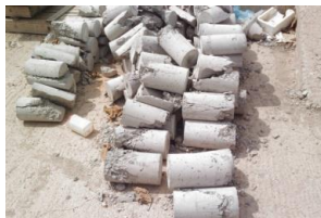
Figure 3. Cylinder of parent concrete after compression failure
