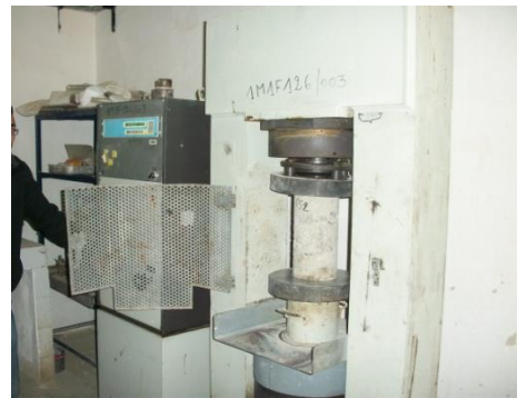
Figure 9. Compression test of large concrete cylinders
