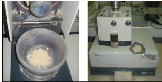
Fig. 3. The grinder used to mixing Clay matrix and PEG 6000 [4]
