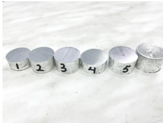
Figure 3. Al 2 O 3 nanofibers/Al composite
