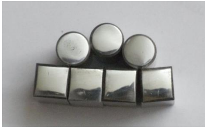
Figure 5. The square and cylindrical pins before coating
