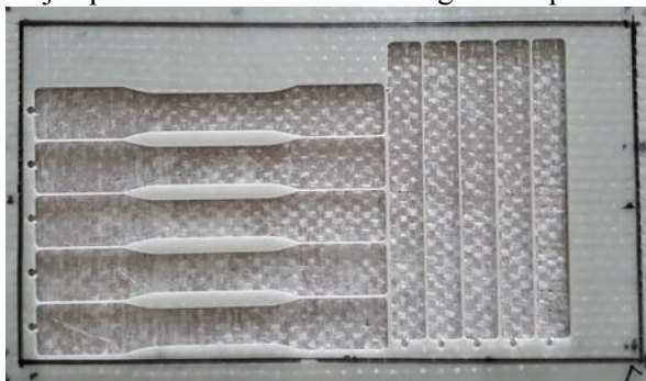
Figure 1. Laminate cutting scheme
