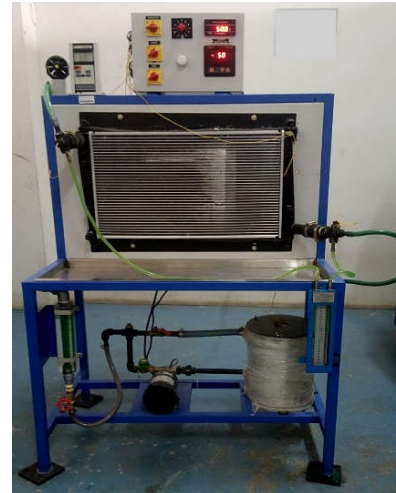
Figure 2 Radiator Test Rig
