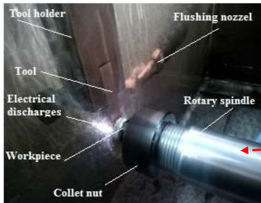
Figure 1. The idea of EDT process.
