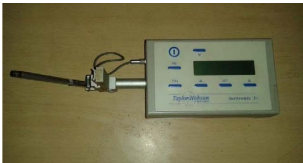
(a) Taylor/Hobson Surtronic 3+ surface roughness tester
