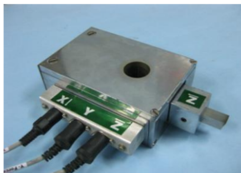
Fig 2.1: lathe tool dynamometer
