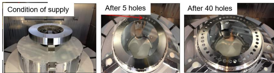
Figure 2: Workpart and fixture used in this study
