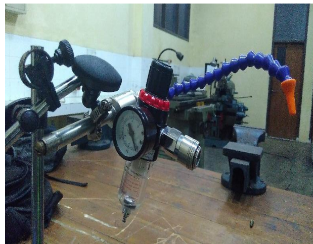
Figure 2. Vortex tube used to produce air cooling.
