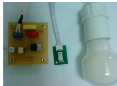
Figure 6. PWM circuit, sensor, and lamp
