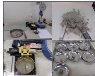
Figure 8. Atterberg limit test.
