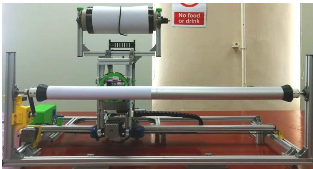
Figure 8. 3-axis filament winding machine.
