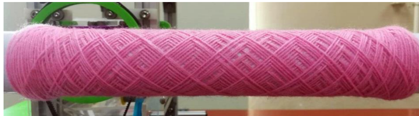
Figure 18. 45° winding angle experiment product with front view.
