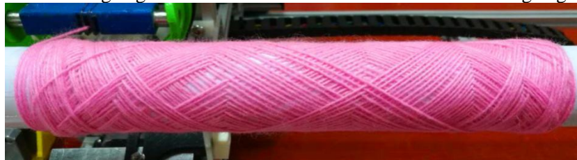
Figure 15. 30° winding angle experiment product with front view.
