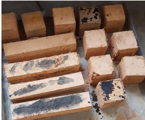
Figure 1. Cube and prismatic samples ready for testing (cubes size: 150 mm × 150 mm × 150 mm; prismatic specimens Size 100 mm × 100 mm × 500 mm)
