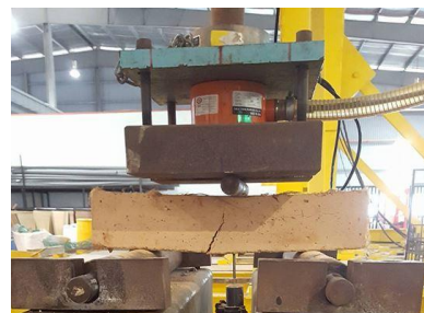
Figure 4. A prismatic sample being tested for flexural strength
