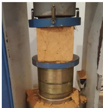
Figure 3. A cube sample being tested for compressive strength
