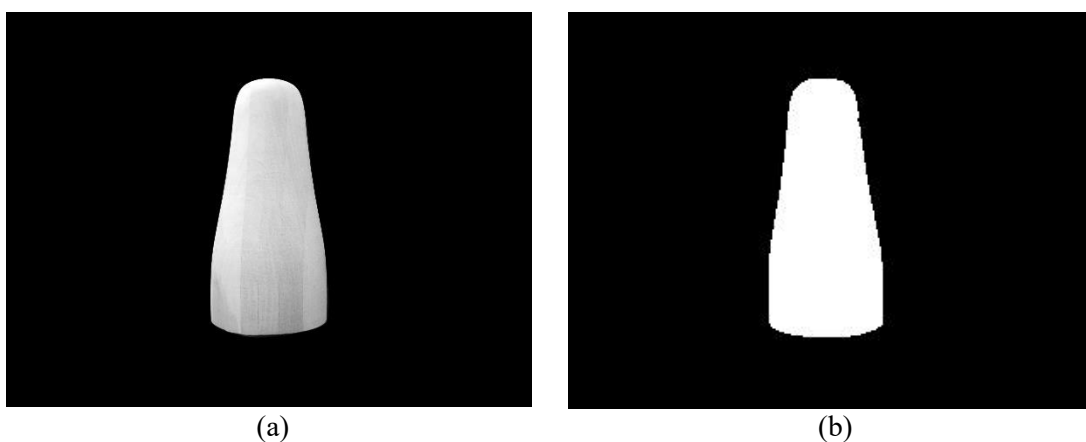
Figure 4. Image of an object (a) before and (b) after Otsu thresholding.
