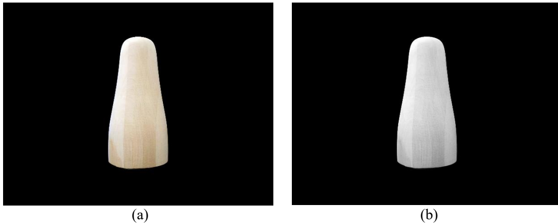
Figure 3. Image of an object (a) before and (b) after grey-scaling.
