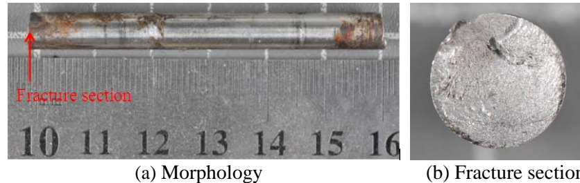
Figure 3. Morphology and fracture section of teeter pivot bolt
