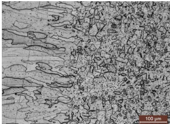
Figure 2. Microstructure of weld interface
