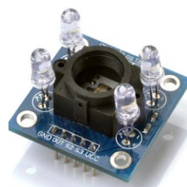
Figure 2. Sensor TCS3200
