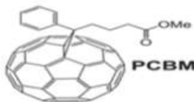
Figure 2. PCBM Structure (Bahtiar, A., et al. 2011).
