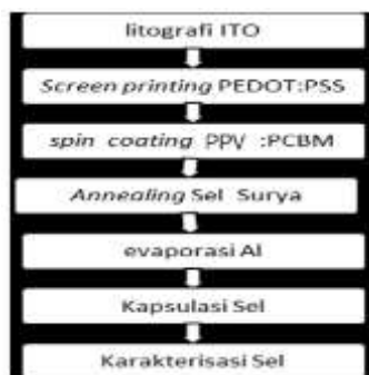
Figure 3. Flow chart of PCBM polymer solar cell research procedure: PPV
