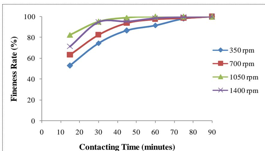
**Figure 1.** Effect of four-blade turbine configuration on fineness rate at agitator speed variation.
