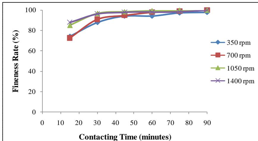
**Figure 3.** Effect of three-blade propeller configuration on fineness rate at agitator speed variation.
