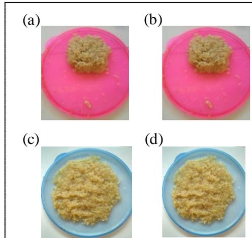
**Figure 2.** Cut material fineness rate at 90 minutes, four-blade turbine type. (a) 350 rpm (b) 700 rpm (c) 1050 rpm (d) 1400 rpm.
