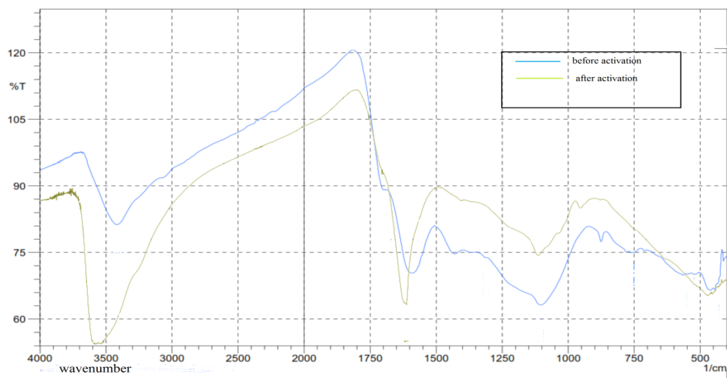
Figure 1. FTIR spectra of sawdust charcoal before and after activation
