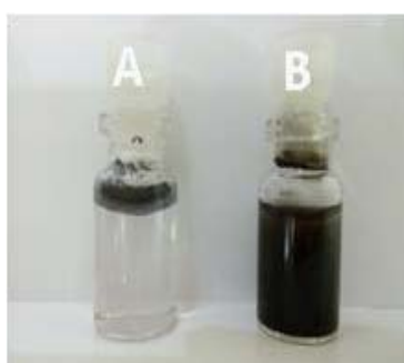
Figure 5. Dispersion test of (A) unmodified \text{Fe}_3\text{O}_4/\text{C} produced using submerged arc discharge in ethanol only (B) and amine-modified \text{Fe}_3\text{O}_4/\text{C} produced using submerged arc discharge in ethanol/ethylenediamine.
