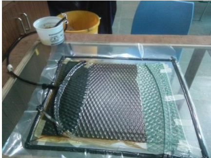
Figure 6: Vacuum Assisted Resin transfer moulding
