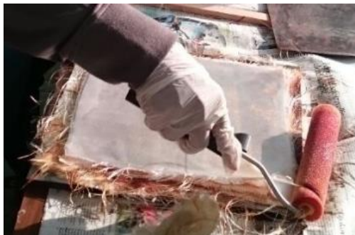
Figure 2: Hand layup process
