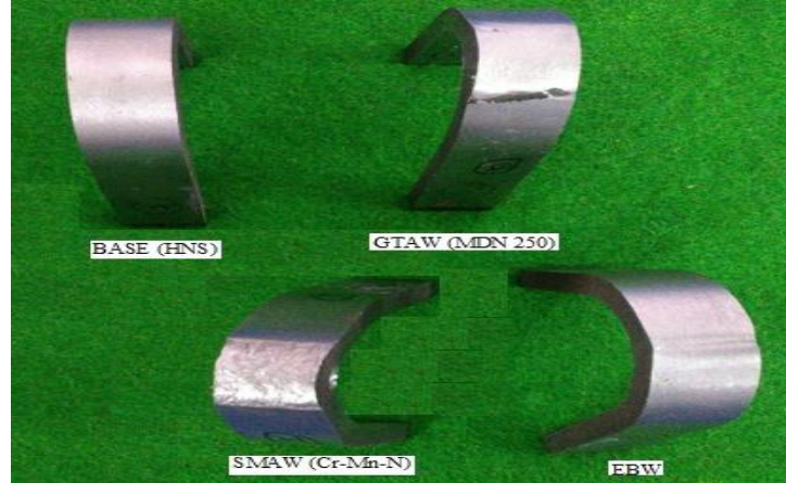
Fig. 15 Face Bend Specimens of nickel free high Cr-Mn-N steel welds
