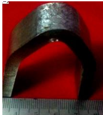
Fig. 13 Face bend ductility test specimens of shielded metal arc weld of nickel free high nitrogen stainless steel
