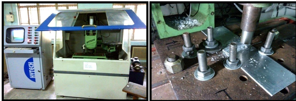
Figure 2: Experimental set up used for making FSW joint [CAM lab, MED, B.I.E.T. Jhansi]
