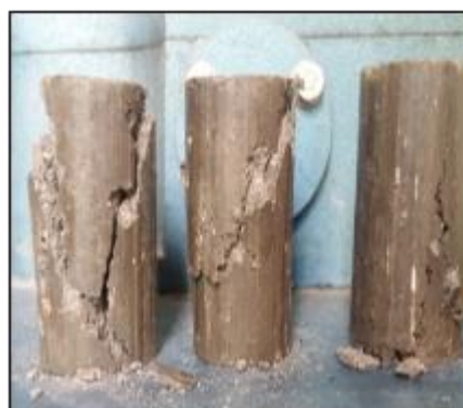
Figure 5 Failed specimens after UCS test showing shear failure
