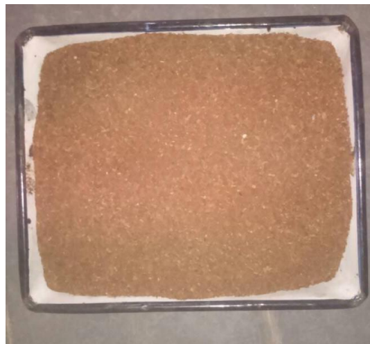
Figure 2 Photograph of the coir pith sample passing 4.75mm IS sieve after air drying
