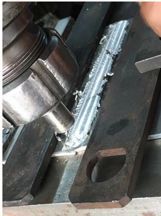
Figure 3. Material Clamping and FSW process
