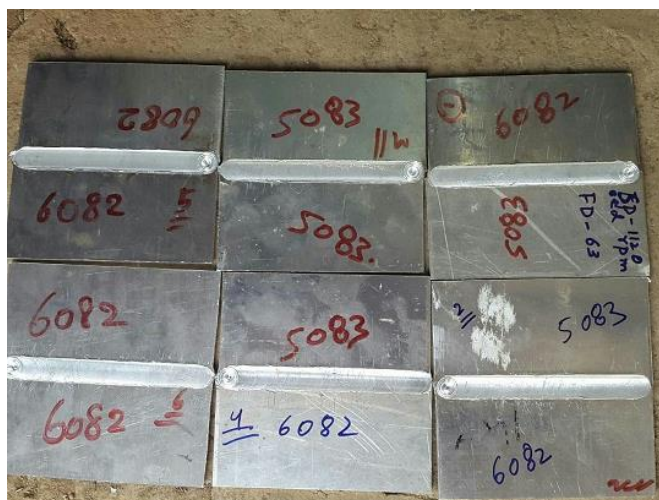
Figure 1. Fabricated Similar & Dissimilar Aluminum Alloys
