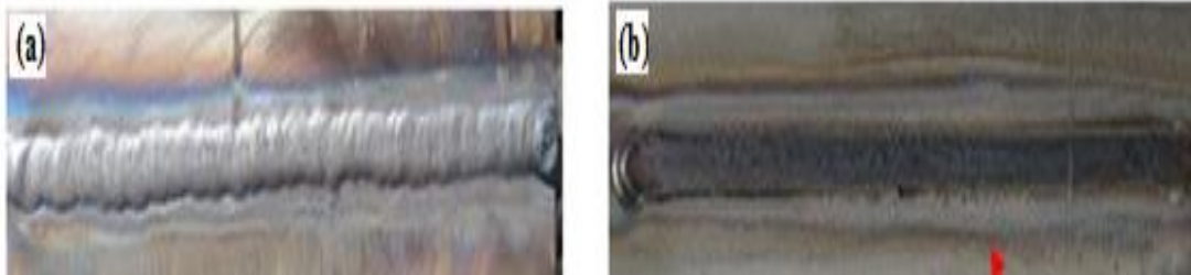
Fig. 1 DSS 2205 Welded plate (a). GTAW and (b) A-GTAW
