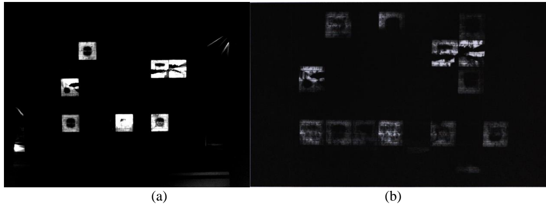
Fig.3 EL images of modules from the PV system. (a) before positive bias PID test, (b) after positive bias PID test
