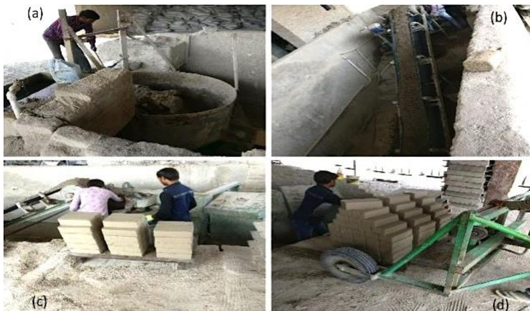
Figure 4. Steps for fly ash bricks construction in a manufacturing unit.
