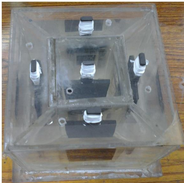
Figure 4. Photograph of a multi chamber MFC fabricated by Samsudeen N et al [22]
