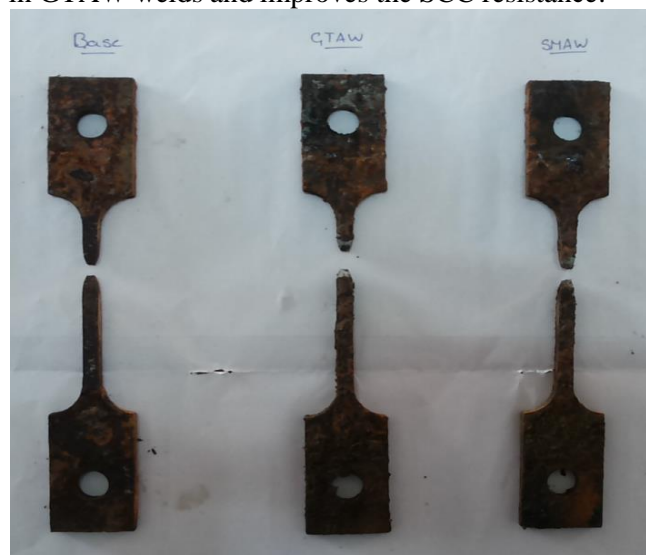
Fig. 10 Failed SCC specimens of DMR 249A and its welds
