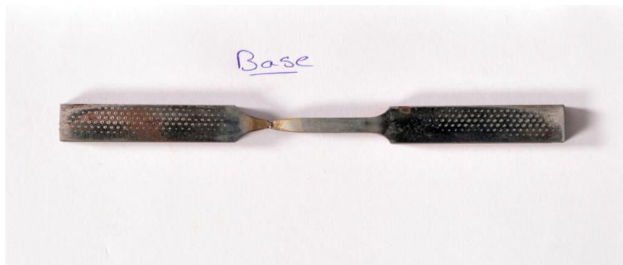
Fig. 4 Failed tensile specimen of Base metal (DMR 249A)
