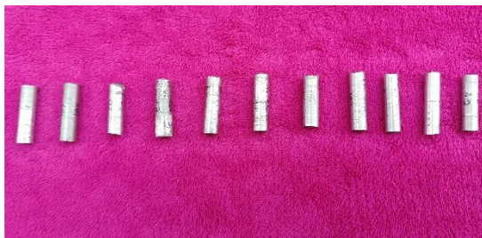
Fig. 2a AA6061-AlNp Pins after testing
