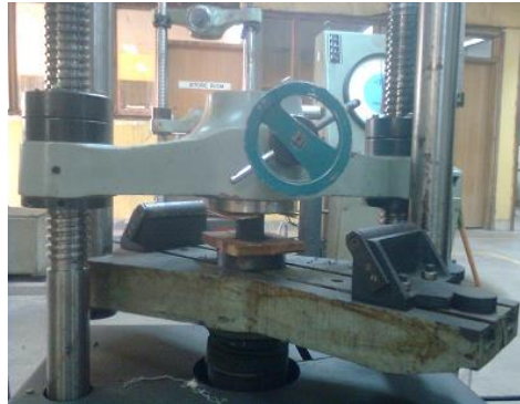
Fig.4 Cold Crushing Strength (CCS) testing
