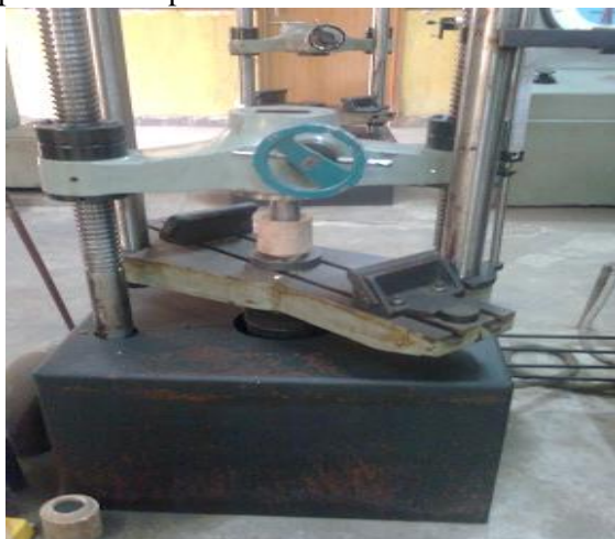
Fig.5 Sample pressing inside refractory tube
