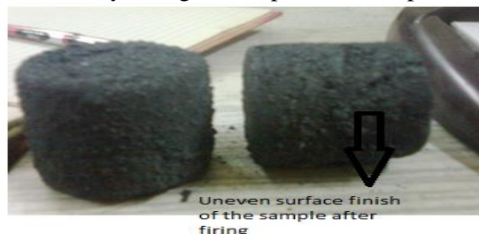
Fig.9 Fired fly ash Tap Hole Clay (THC) samples
