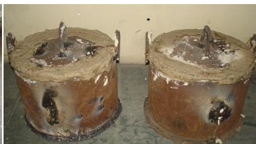
Fig.3 Samples packed in container for firing
