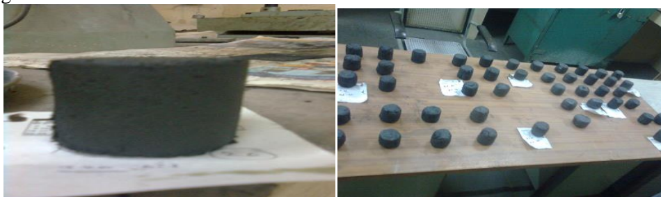
Fig. 1 Prepared tap hole clay samples
