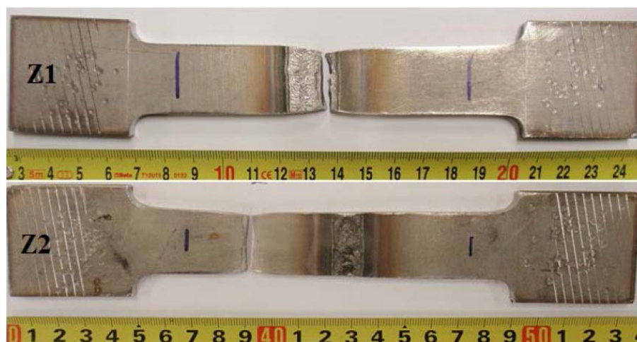
Figure 6. Testing samples after transversal tensile testing [9]
