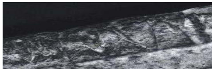
Figure 2. Bright field image TEM of AlN thin film microstructure after annealed at temperature of 1500 °C.
