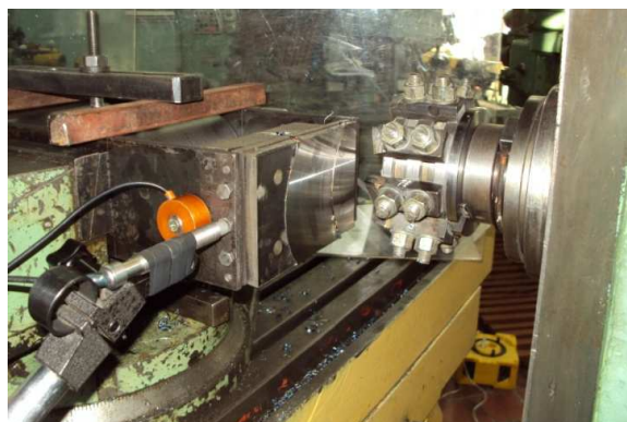
Figure 2. An experimental unit with a fixture for creating a low-rigidity workpiece in a feed direction
