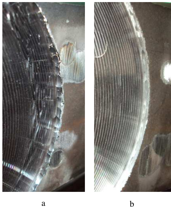
Figure 6. Machined surface and workpiece cutting surface when machining with a constant teeth-pitched mill (a) and a variable alternative teeth-pitched mill at a difference of 8^\circ (b)
