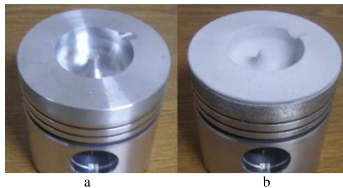
Figure 4. Unprotected piston (a) and protected one (b) by semitransparent PSZ- ceramics.
