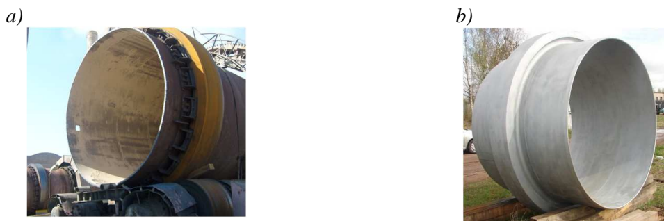
Figure 1. Design of rotary TD supports: a) “F” tyres; b) “W” tyres
