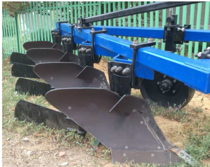
Figure 3. Industrial prototype of plow with complete turnover of soil layers
