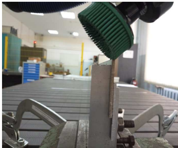
Figure 2. 3M Scotch-Brite Roloc Bristle P50 tool adjustment for edge machining
