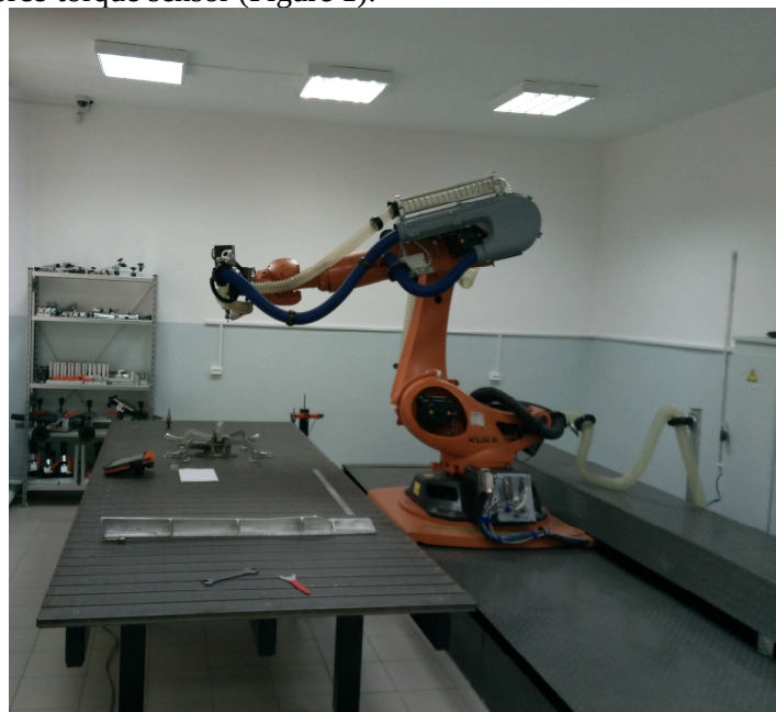
Figure 1. Robotic center for edge machining
