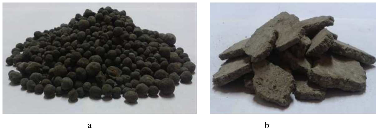
Figure 1. Clinker: a - initial material, b – material after milling in a PRG.
